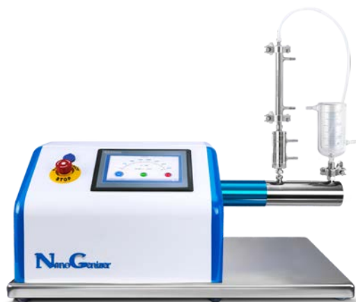
Inlet Reservoir: Jacketed Glass Cylinder
